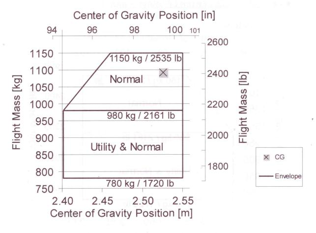
The CG shown in the diagram is that from the example in Table 6.4.3 (b) CALCULATION OF LOADING CONDITION, row 7 (pre take-off condition).
