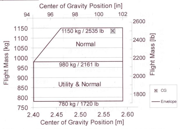
The CG shown in the diagram is that from the example in Table 6.4.3 (a) CALCULATION OF LOADING CONDITION, row 7 (pre take-off condition).
